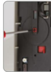
*The Easy Adjust system available on the MASTER 12.8 PLUS AJ, enables to adjust in a simple and effective way tanks to a simply turning a screw the orientation compared with the ground of the beams generated by one of the two passive infrared. This enables you to configure the coverage area of the detector in a timely manner.*
